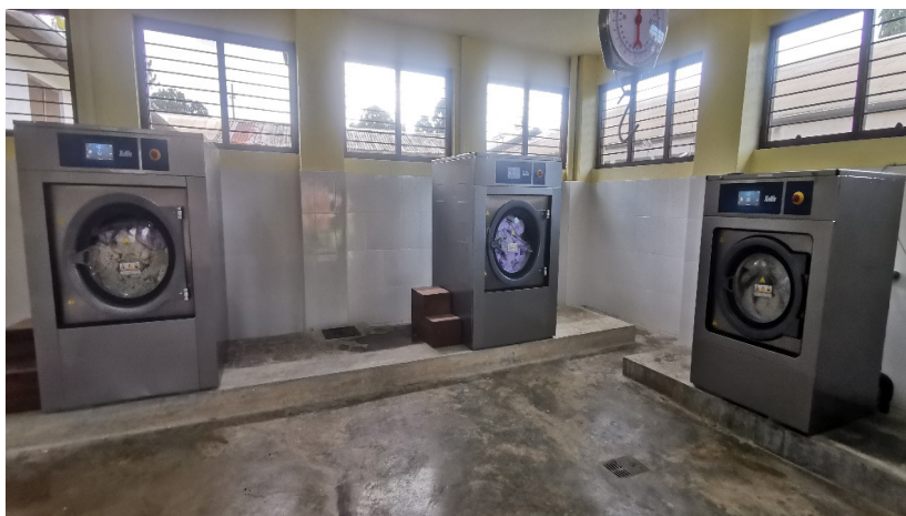
Picture: 3 New Washing Machine (2 on the left 45Kg, 1 on the Right 25Kg) All machines are connected on the hospital network can be seen and monitored remotely for troubleshooting their problems and checking their performance easily
